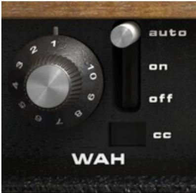
What if you don't have any continuous controller on your keyboard? Well, we thought of that and modeled an auto-wah feature. Unlike other auto-Wah that opens when detecting an attack, ours was designed after what really happens on a real one. Its frequency can be changed and also synched to the tempo if needed.
