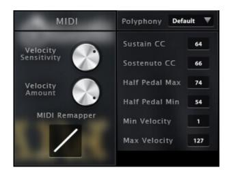
Included in the V3 update are some MIDI controls. The sostenuto and sustain CC can be adjusted to suit the use of an expression pedal instead of a regular on/off pedal. You can also alter the MIDI curve, the dynamics and the velocity response to refine the library to your taste, keyboard and playing style.
