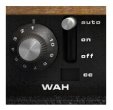
What if you don't have any continuous controller on your keyboard? Well, we thought of that and modeled an auto-wah feature. Unlike other auto-Wah that opens when detecting an attack, ours was designed after what really happens on a real one. Its frequency can be changed and also synched to the tempo if needed.
